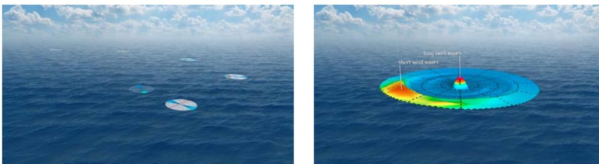
Fig. 6.1b. Step 2: the 1D-radar reflectivity modulations are determined for each footprint, to provide directional spectral information, at Level-2b\_WDS, and a 2D wave spectrum is retrieved at Level-2c by combining 1D spectra over a 70×70 km grid cell. (ESA/Planetary Visions)
