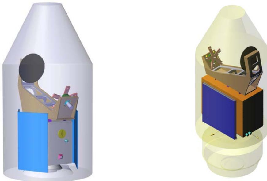
Figure 5.52. Accommodation of SKIM in the Vega-C fairing on top of short VESPA-C, Concept A (left) and Concept B (right).
