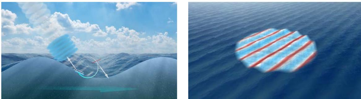
Fig. 6.1a. Step 1: Doppler velocity and roughness modulation measurements are made at Level-1b radar footprints across the SKaR instrument swath with different angular and beam elevation diversity. (ESA/Planetary Visions)
